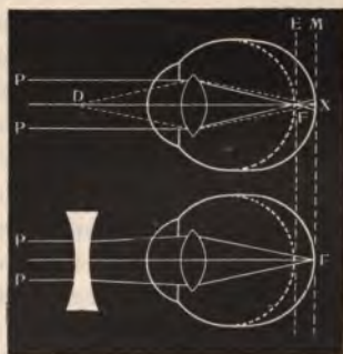
FIG. 192.—The Focussing of Parallel and Divergent Rays in Myopia.
